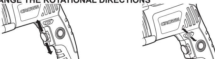
Operate the rotation direction switch only at a standstill.
